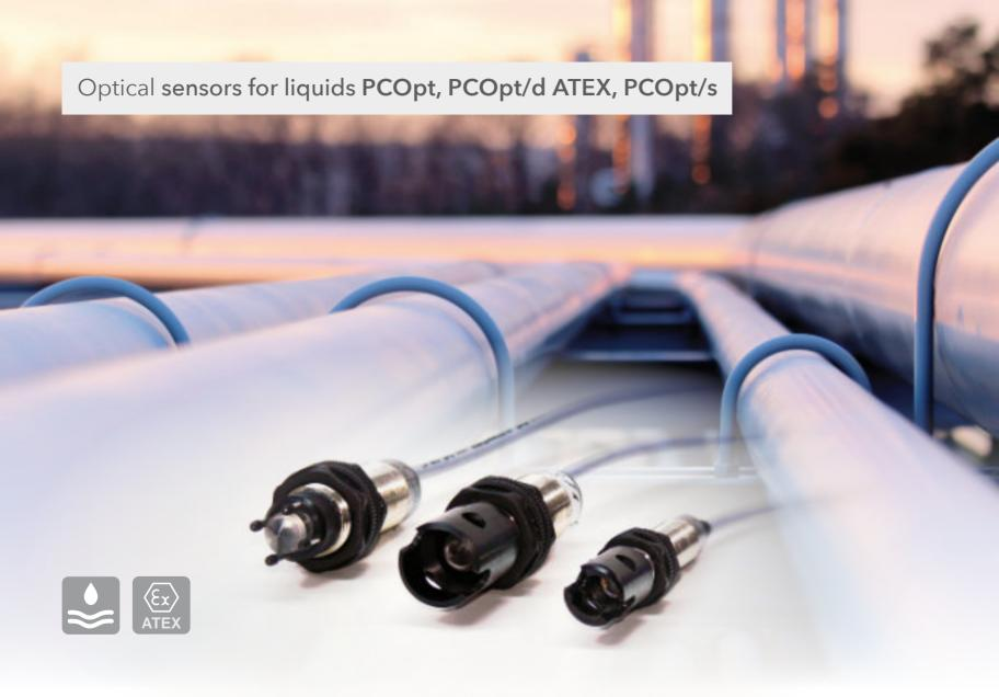
**PCOpt - optical sensor for liquids,** basic sensor that detects appearance or disappearance of any kind of liquid. Used in "wet" detection systems, can be placed in piezometers at one-mantle tanks, in the vicinity of pipelines or in the space between the mantles of two-mantle tanks.
