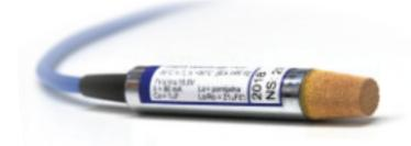
PCO - vapor sensor for oil-derivative products, most popular sensor for leak detection systems. Used in "dry" detection systems, can be placed in piezometers at one-mantle tanks, in the vicinity of pipelines or in the space between the mantles of two-mantle tanks. It can also be located on any dry base.
